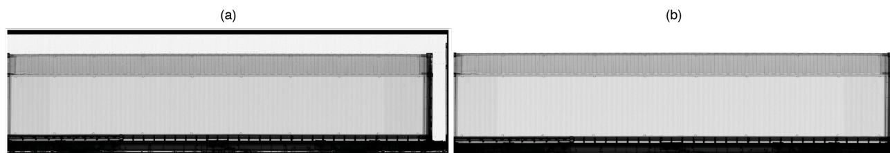
Figure 1. Example of preprocessing: (a) the raw SoC X-ray transmission image, and (b) the SoC X-ray transmission image having been preprocessed .
